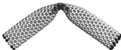
FIGURE 4.9 MD simulation of a large-amplitude transverse deformation of a carbon nanotube, apparently beyond the elastic limit. In fact, the tube snaps back once the computer-generated force is removed, and there is no plastic deformation or permanent damage. (From Yakobson, B. I., Appl. Phys. Lett. 72 , 918–920 (1998), with permission.)
